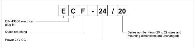
The ECF connector is a digital amplifier controlling open loop on-off valves.
