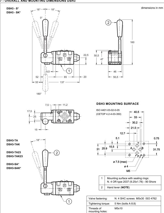
NOTE: The valve is supplied with the hand lever oriented in a perpendicular position with respect to the mounting surface (as indicated in the above drawing). For installation needs the hand lever can be oriented by the user directly at 180° to the standard position, simply by unscrewing the lever and re-screwing it in the desired position.
