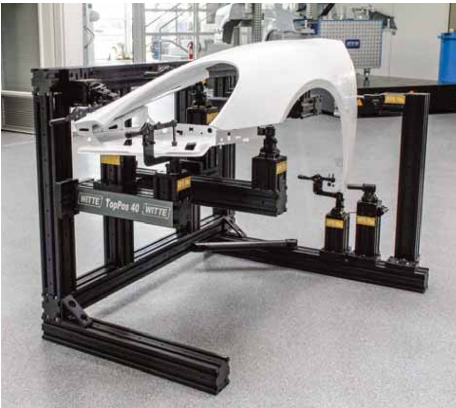
Fixture for fender in frame style
